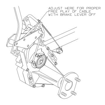
**NOTE:** Cable must have the recommended 1-1/2 to 2 inches of free play with parking brake released or drive belt may slip, causing loss of power.
